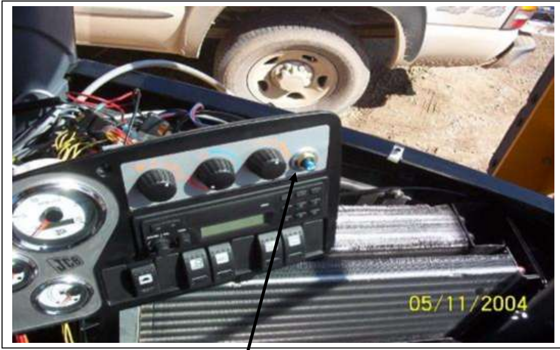
Mount A/C on-off push button switch in existing hole in metal panel behind decal.
