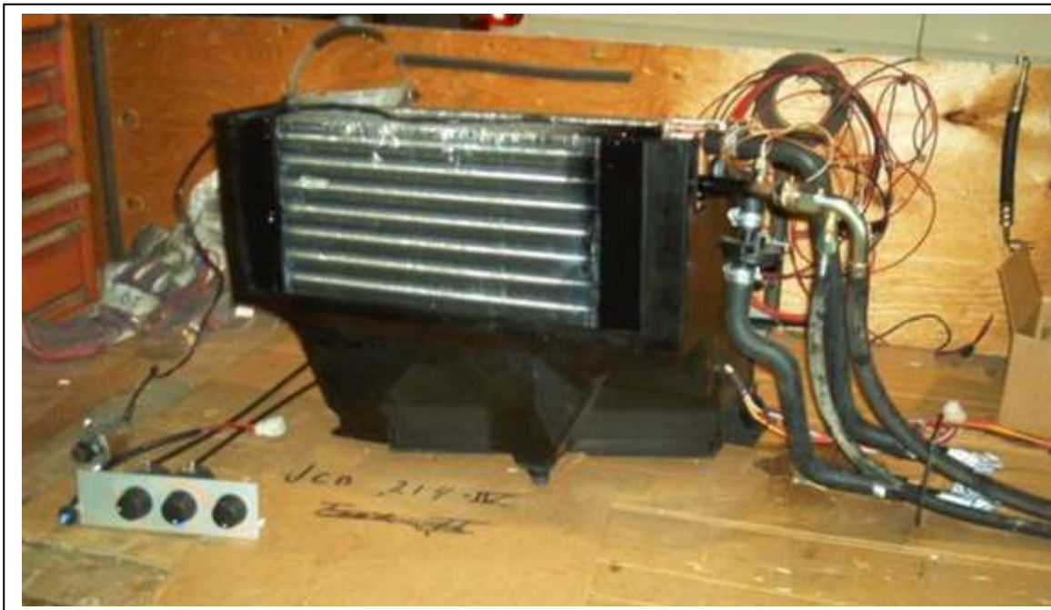
Fitting connections shown at evaporator coil with box out of machine. *NOTE: Do not take box out.**
