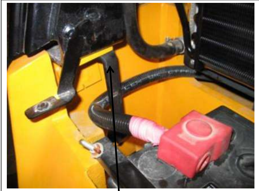
Bolt 90 0 drier bracket using existing M10 bolt here on older machines.
