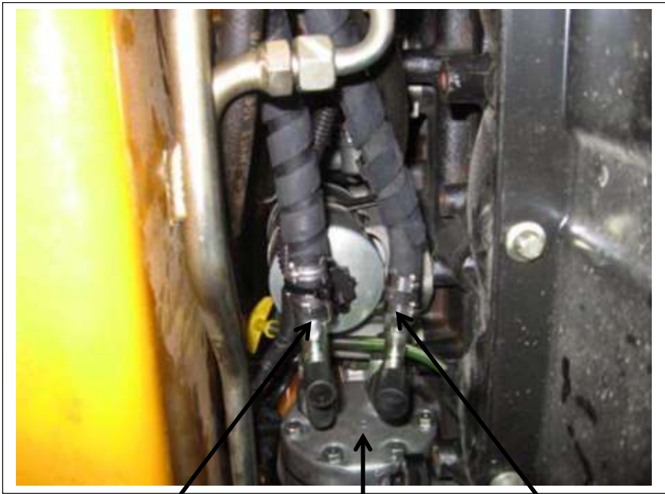
1/2" line at compressor
