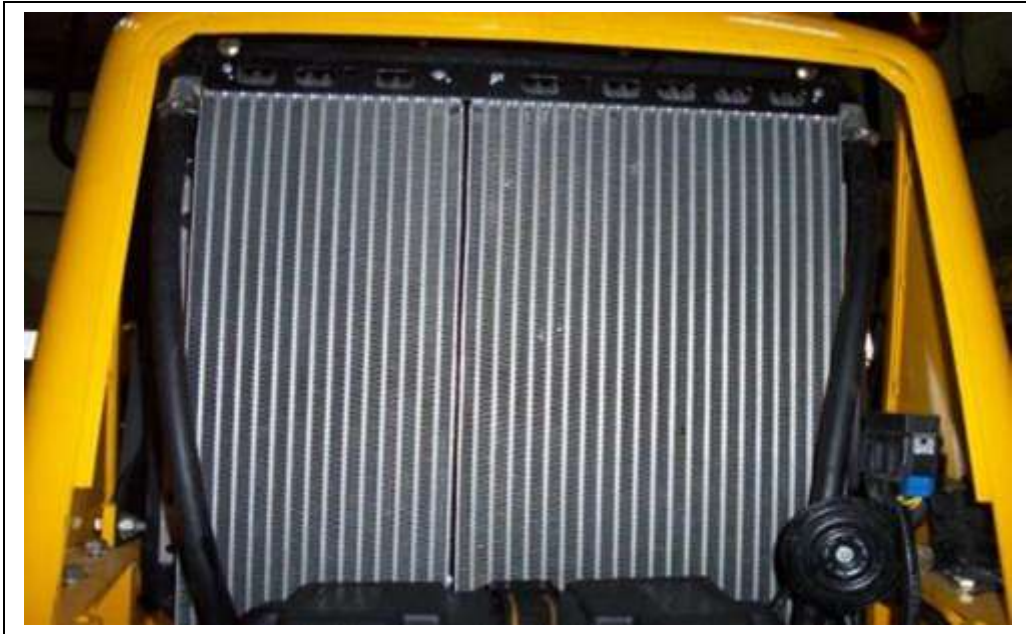
Remove radiator front grill
