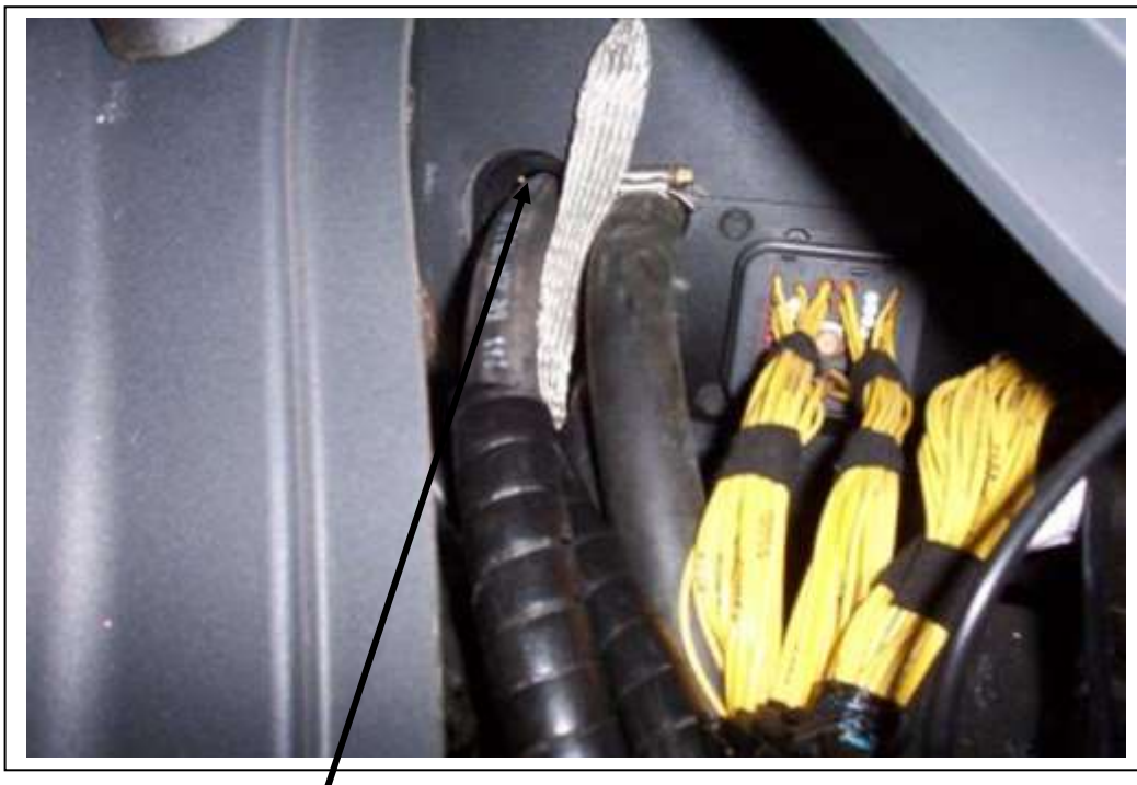
A/C lines passing through existing holes beside heater lines. *NOTE: the fittings cannot be installed on these hoses until they have been put through these holes.*
