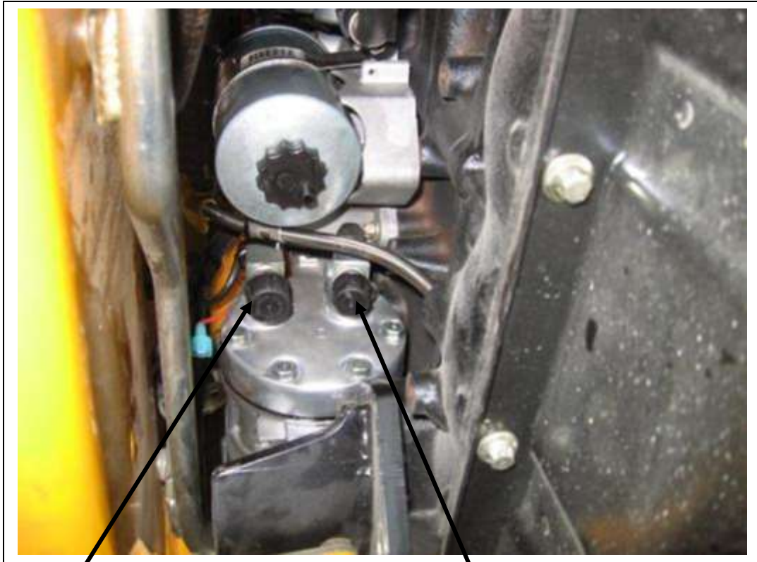
1/2" rotolock fitting on suction side
