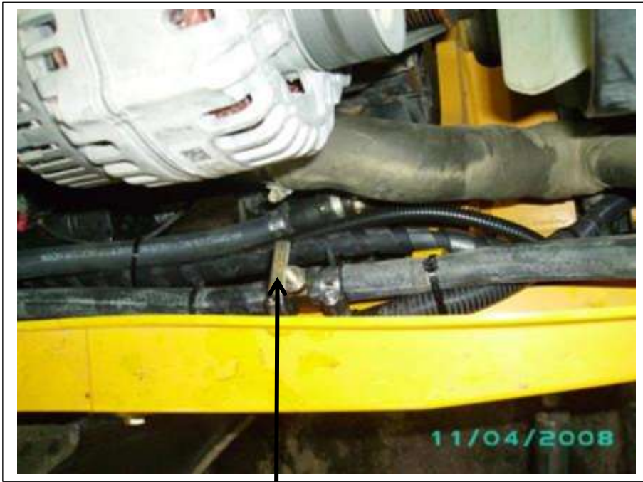
Heater shut off tap installed in one heater line. Exact position varies depending on the age of the machine.
